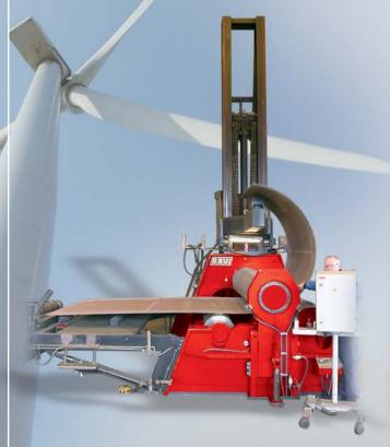
Front, rear and overhead supports (self-aligning for cones) adjust for the cone being rolled for added safety and stability
