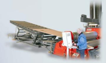
When prebending the leading edge, the conveyor supports the plate (no crane!)
