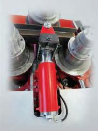
H, U and I beams bent the-hard-way require a special traction unit to pull the profile downward during the rolling process. It is hydraulically activated and is controlled through the operator panel. The traction unit position is easily adjustable. Davi can provide rolls for this traction unit customized to any beam to be bent.
