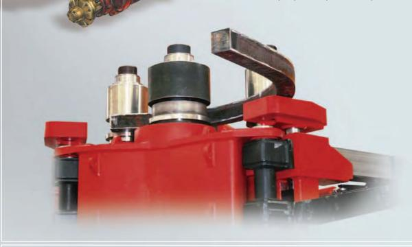
The guide rolls are the strongest in the industry, and hydraulically activated on all DAVI MCP. All six movements (In-out / up-down /tow-away) are therefore controlled from operator panel, resulting in high performance and a quicker production time.
